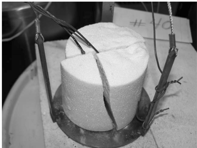
Figure 2. Resulting fractured cylinder from test 40C.
